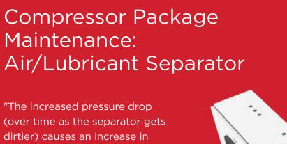
(over time as the separator gets dirtier) causes an increase in compressor airend discharge pressure, with a resulting increase in power. If electricity prices are high, replacing the separator before the pressure drop reaches 10 PSI will reduce energy costs."
